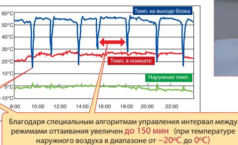
**Пример эксплуатации наружного блока**
